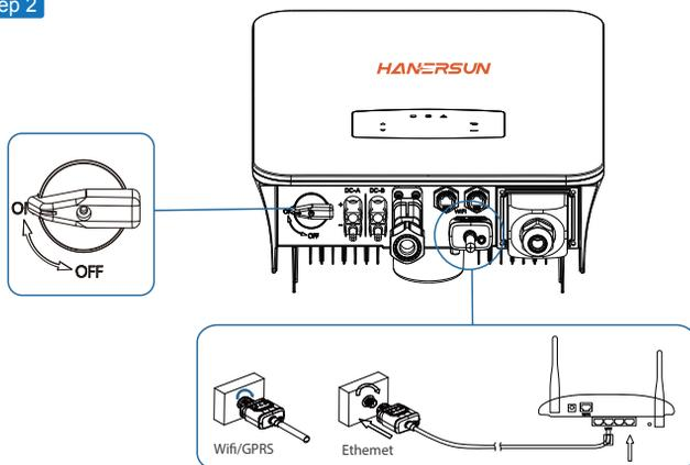
Turn on the DC switch and AC circuit breaker, and wait until the LED indicator on the monitoring module flashes, indicating that the monitoring module is successfully connected.
