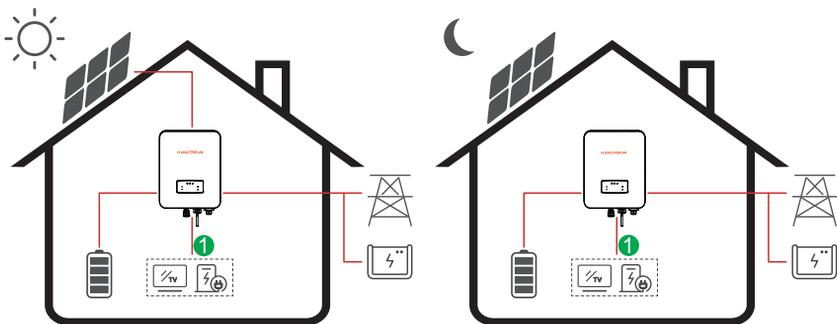
**Energy flow:** PV and Battery → Load
