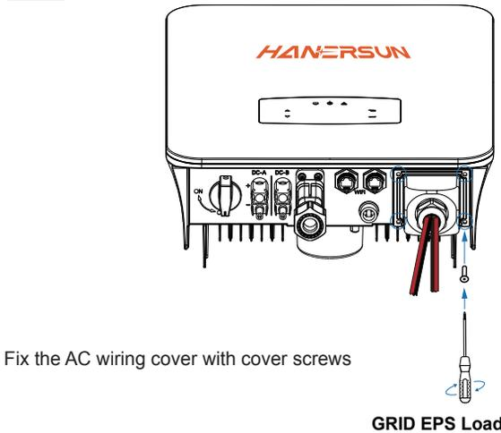
Fix the AC wiring cover with cover screws
