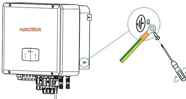
Fix the grounding screw to the grounding connection of the machine housing.
