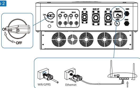
Turn on the DC switch and AC circuit breaker, and wait until the LED indicator on the monitoring module flashes, indicating that the monitoring module is successfully connected.
