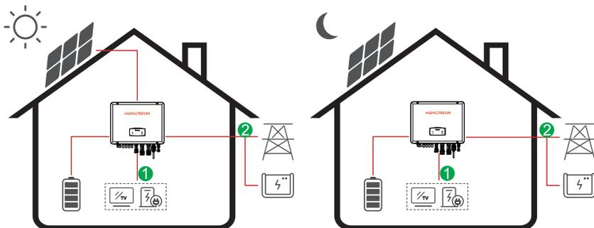
Energy flow: Battery and PV → Load → Grid
